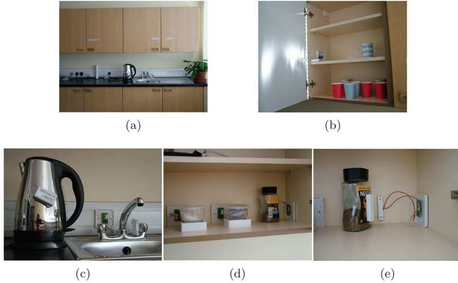
Fig. 1: Sensors within smart kitchen environment to assess the ADL of preparing a drink (a) picture of the semi-functioning kitchen, (b) cupboard with door sensor, (c) kettle with tilt switch and contact switch on tap, (d) contact sensors on sugar, tea and coffee jar and (e) contact sensor on coffee in 'on' state
