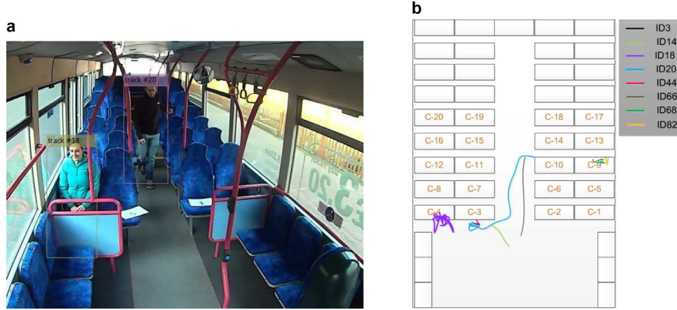
Fig. 6. Outputs of the tracker: (a) image with tracker bounding boxes over the person in the scene; (b) the corresponding track plots in real-world coordinates.
