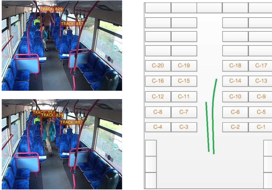
Fig. 10. Sequence 8—top-left: image of male moving close to seat 18; bottom-left: image of female moving away from seat 11, towards the bus door; right: trajectory corresponding to PM event E127 detected by a tracker—TRACK 829.
