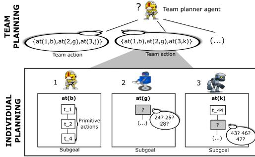
Fig. 3: Actions and subgoals: a team action is associated one or more subgoals, each of which indicates (in our scenario) a target location to be reached e.g.  $at(k)$ , whereas primitive actions indicate trails to be crossed, e.g.  $t_{44}$ .
